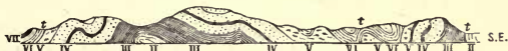
Section from the Great North to the Little North Mountain through Bore Springs, Va.; t, t, position of thermal springs; II, Calciferous formation; III, Trenton; IV, Hudson River; V, Oneida; VI, Clinton and Lower Helderberg; VII, Oriskany Sandstone and Cauda-Galli Grit.
